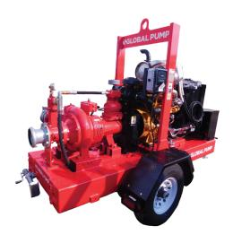
Global Pump® High Performance Trash pumps are specifically designed to effectively handle a wide-range of liquids from water to sewage and sludge that can contain solids and other material.
