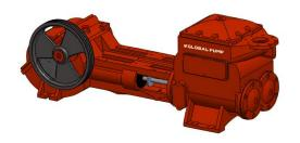
**PUMP MATERIAL** Cast Iron Pump Liquid End **Brass** Valve Seat, Weight, Spring & Washer Valve **NBR Gear Casing** SG Cast Iron Valve Stem 304 Stainless Steel Cylinder Liner 316 Stainless Steel Leather Piston Cup Piston Rod 304 Stainless Steel Piston Rod Seal Gland Packing Skid & Frame Hot Dipped Galvanized Steel Roof, Panels & Doors Steel Fuel Tank Steel
